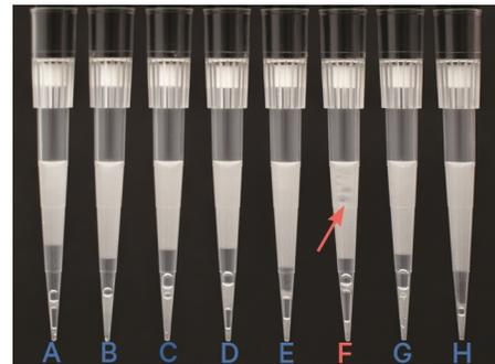
In pipette tips A-E & G-H, a portion of the emulsion displays separate layers of oil, which indicates clog. Pipette tip F indicates a clog (separate oil layers) and wetting failure (non-uniform emulsion).
