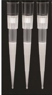
All liquid levels are similar in volume and opacity without air trapped in the pipette tips.
