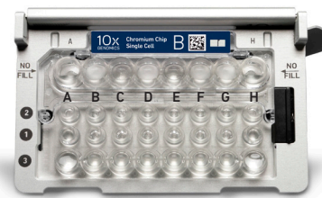
Recovery Well G indicates a reagent clog. Recovery Well C and E indicate a wetting failure. Recovery Wells B, D, and F are normal. Wells A and H contain 50% Glycerol Solution.
