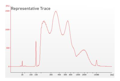
**b. OR** Run **2**  $\mu$ l sample on the Agilent TapeStation D1000 ScreenTape to determine fragment size.
